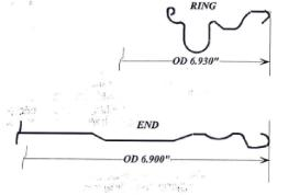
DESCRIPTION: Round steel can with a welded side seam and a multiple friction closure.
