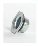
The metal plug VGII has an electro zinc chromate finish, rounded bottoms, and wide shoulders with concentric sealing beads to help lock gaskets securely into place. Known for it's distinctive flathead surface, the metal plug has no crossbar or dome features. This fitting is available in Zinc Plated or Buff Epoxy with White EDPM, Black Buna, or Poly Irradiated Gaskets. A Red Phenolic option is also available.
