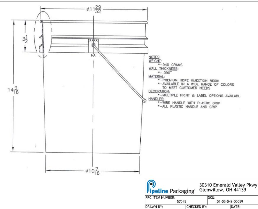
11/27/2018 DESCRIPTION: COLOR: PROPRIETARY AND CONFIDENTIAL **UNLESS OTHERWISE SPECIFIED:** 5 Gal HDPE Gray Open Head Pail THE INFORMATION CONTAINED IN THIS DRAWING IS THE SOLE UNITS OF MEASURE: Inches PART MATERIAL: **VOLUME:** WEIGHT: PROPERTY OF PIPELINE PACKAGING. ANY REPRODUCTION IN PART OR AS A WHOLE WITHOUT THE WRITTEN PERMISSION OF DWG SIZE: DWG NO.: SHEET NO: REV: TOLERANCES: Specified in drawing PIPELINE PACKAGING IS PROHIBITED. Α 1 of 1
