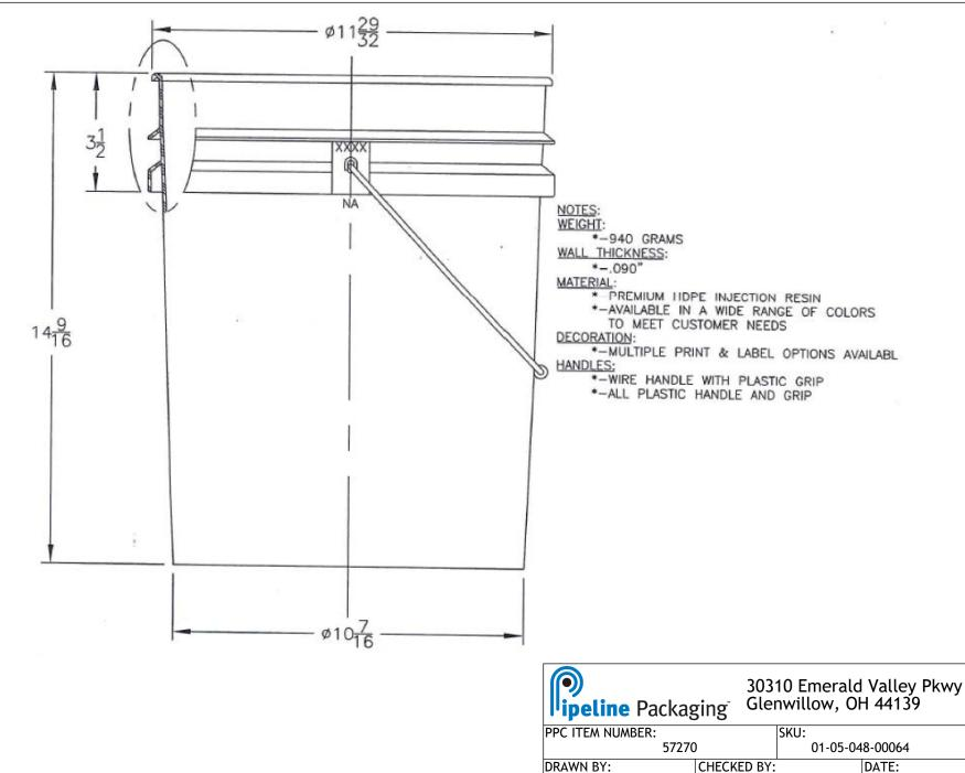
11/27/2018 DESCRIPTION: COLOR: PROPRIETARY AND CONFIDENTIAL **UNLESS OTHERWISE SPECIFIED:** 5 Gal HDPE Yellow Open Head Pail THE INFORMATION CONTAINED IN THIS DRAWING IS THE SOLE UNITS OF MEASURE: Inches PART MATERIAL: **VOLUME:** WEIGHT: PROPERTY OF PIPELINE PACKAGING. ANY REPRODUCTION IN PART OR AS A WHOLE WITHOUT THE WRITTEN PERMISSION OF DWG NO.: DWG SIZE: SHEET NO: REV: TOLERANCES: Specified in drawing PIPELINE PACKAGING IS PROHIBITED. Α 1 of 1
