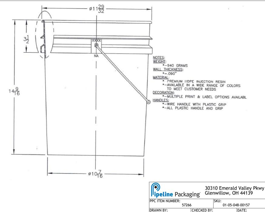
11/27/2018 DESCRIPTION: COLOR: PROPRIETARY AND CONFIDENTIAL **UNLESS OTHERWISE SPECIFIED:** 5 Gal HDPE Blue Open Head Pail THE INFORMATION CONTAINED IN THIS DRAWING IS THE SOLE UNITS OF MEASURE: Inches PART MATERIAL: **VOLUME:** WEIGHT: PROPERTY OF PIPELINE PACKAGING. ANY REPRODUCTION IN PART OR AS A WHOLE WITHOUT THE WRITTEN PERMISSION OF DWG NO.: DWG SIZE: SHEET NO: REV: TOLERANCES: Specified in drawing PIPELINE PACKAGING IS PROHIBITED. Α 1 of 1
