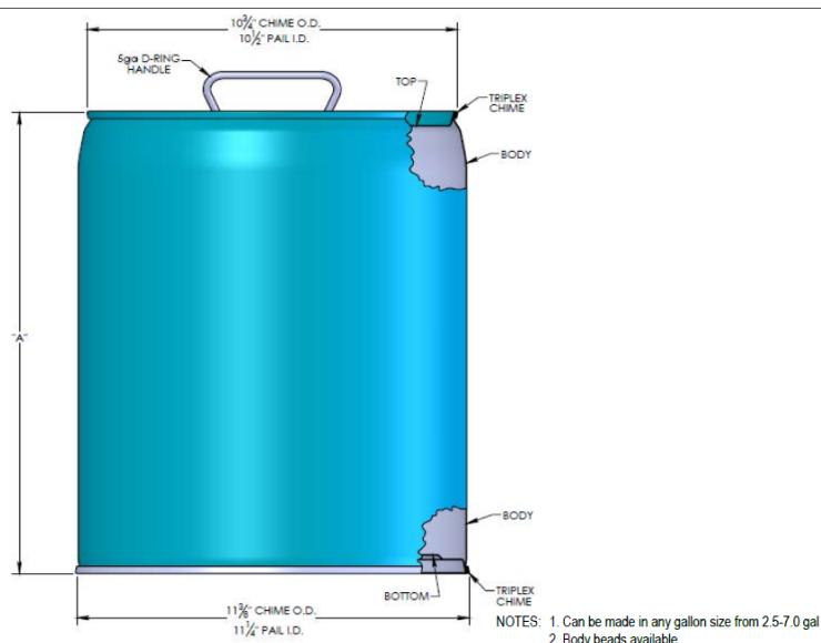
DIMENSION  $2\frac{1}{2}$  3  $3\frac{1}{2}$  4 5 20 L  $5\frac{1}{2}$  6  $6\frac{1}{2}$  7 "A"  $7\frac{3}{8}$ "  $9\frac{1}{16}$ "  $10\frac{3}{16}$ "  $11\frac{5}{16}$ "  $13\frac{7}{16}$ "  $14\frac{1}{2}$ "  $15\frac{5}{16}$ "  $16\frac{1}{8}$ "  $17\frac{1}{4}$ "  $18\frac{3}{16}$ "
