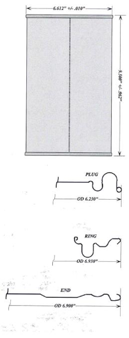
DESCRIPTION: Round steel can with a welded side seam and a multiple friction closure.
