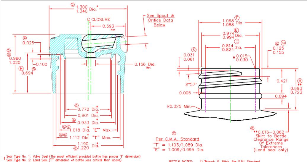
Dimensions marked \* are an average of two measurements taken 90° apart.
