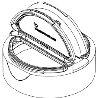
FLAPS IN FULL OPEN DISPENSING POSITION (90°)
