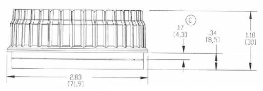
EFFICTIVE "H" DIMENSION IS DETERMINED BY THE TYPE OF LINER USED IN THE CLOSURE. OVERAL "H" WILL BE LESS THAN SHOWN ONCE THE LINER IS APPLIED REFER TO DRAWING M0768-002-A FOR BOTTLE OPENING DETAILS.
