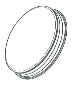
1) A RECESSED STACKING FEATURE INVOLING A RAISED OUTSIDE EDGE IS ACHIEVED BY INCREASING THE HEIGHT OF FLAT TOP CAP BY APPROX. 0.030"
