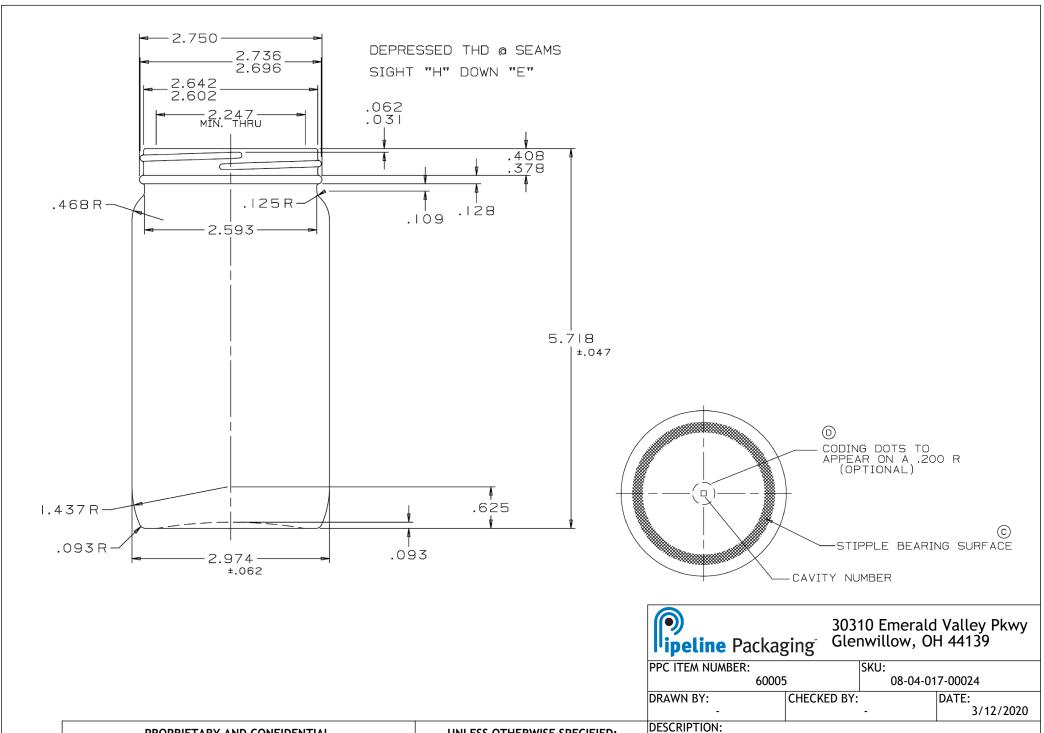
PROPRIETARY AND CONFIDENTIAL **UNLESS OTHERWISE SPECIFIED:** 16 oz Flint Glass AC Jar 70-400 THE INFORMATION CONTAINED IN THIS DRAWING IS THE SOLE UNITS OF MEASURE: Inches PART MATERIAL: **VOLUME:** WEIGHT: PROPERTY OF PIPELINE PACKAGING. ANY REPRODUCTION IN 9.473 oz PART OR AS A WHOLE WITHOUT THE WRITTEN PERMISSION OF DWG NO.: DWG SIZE: SHEET NO: REV: TOLERANCES: Specified in drawing PIPELINE PACKAGING IS PROHIBITED. Α 1 of 1
