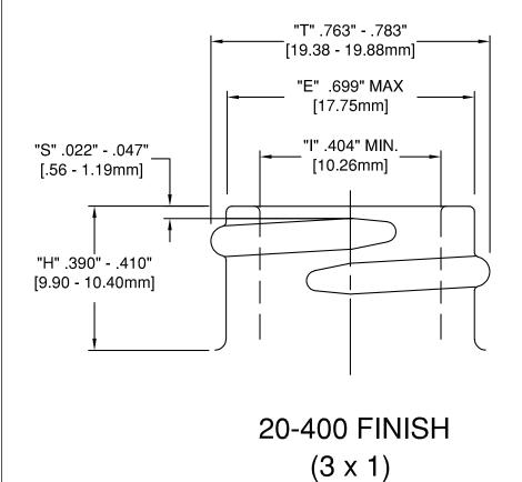
FINISH MUST HAVE MINIMUM OF 1 TURNS OF THREAD WITH FULL PROJECTION
