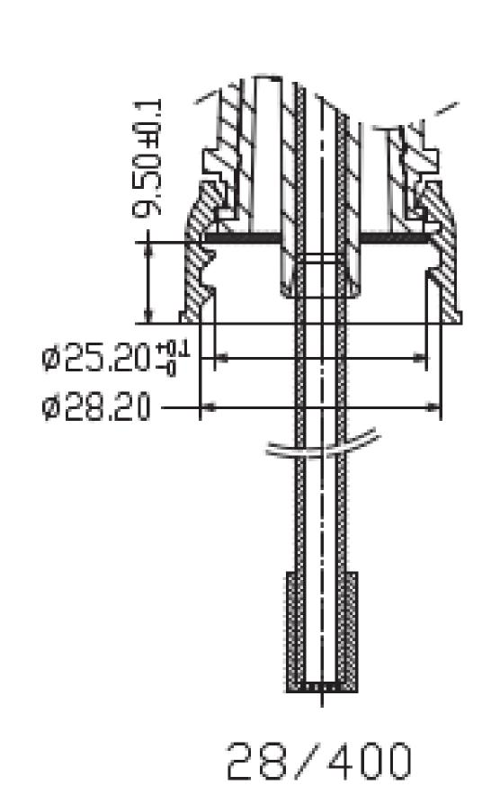
SPRAY DUTPUT PER STROKE  $1.00\pm0.1$ ML
