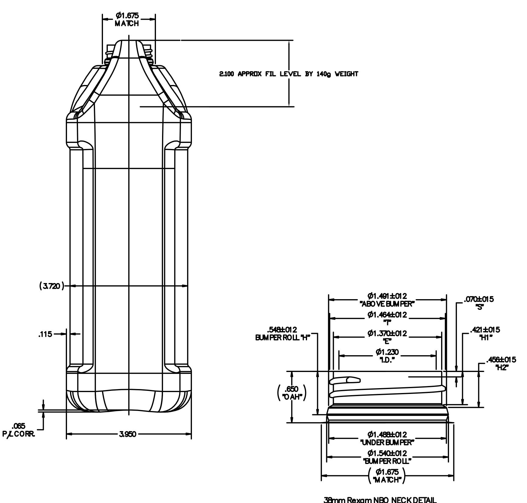
38mm Rexam NBO NECK DETAIL (PER REXAM SPEC # M 6961H)
