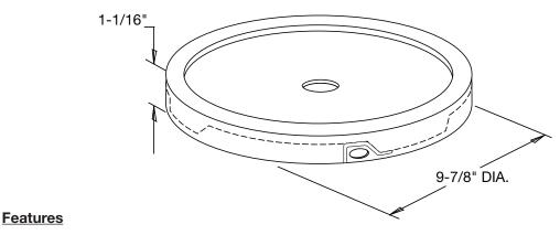
Exclusive four-tab EZ Cover® design EZ to open and reseal Tamper-evident tear-strip Medium duty cover performance Gasketed closure for liquid applications
