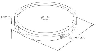
Exclusive four-tab EZ Cover® design EZ to open and reseal Tamper-evident tear-strip Medium duty cover performance Flowed-in gasket (FIG) for dry or liquid applications
