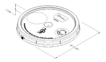
UN – Solids Certified to Y27 / S Tamper-evident tear-strip Medium duty cover performance Tubular EPDM Gasket for all applications
