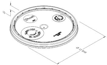
UN – Liquids Certified to Y1.5 / 30 Heavy duty cover performance Tubular EPDM Gasket for all applications
