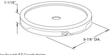
Exclusive four-tab EZ Cover<sup>®</sup> design EZ to open and reseal Tamper-evident tear-strip Medium duty cover performance Gasketed closure for liquid applications
