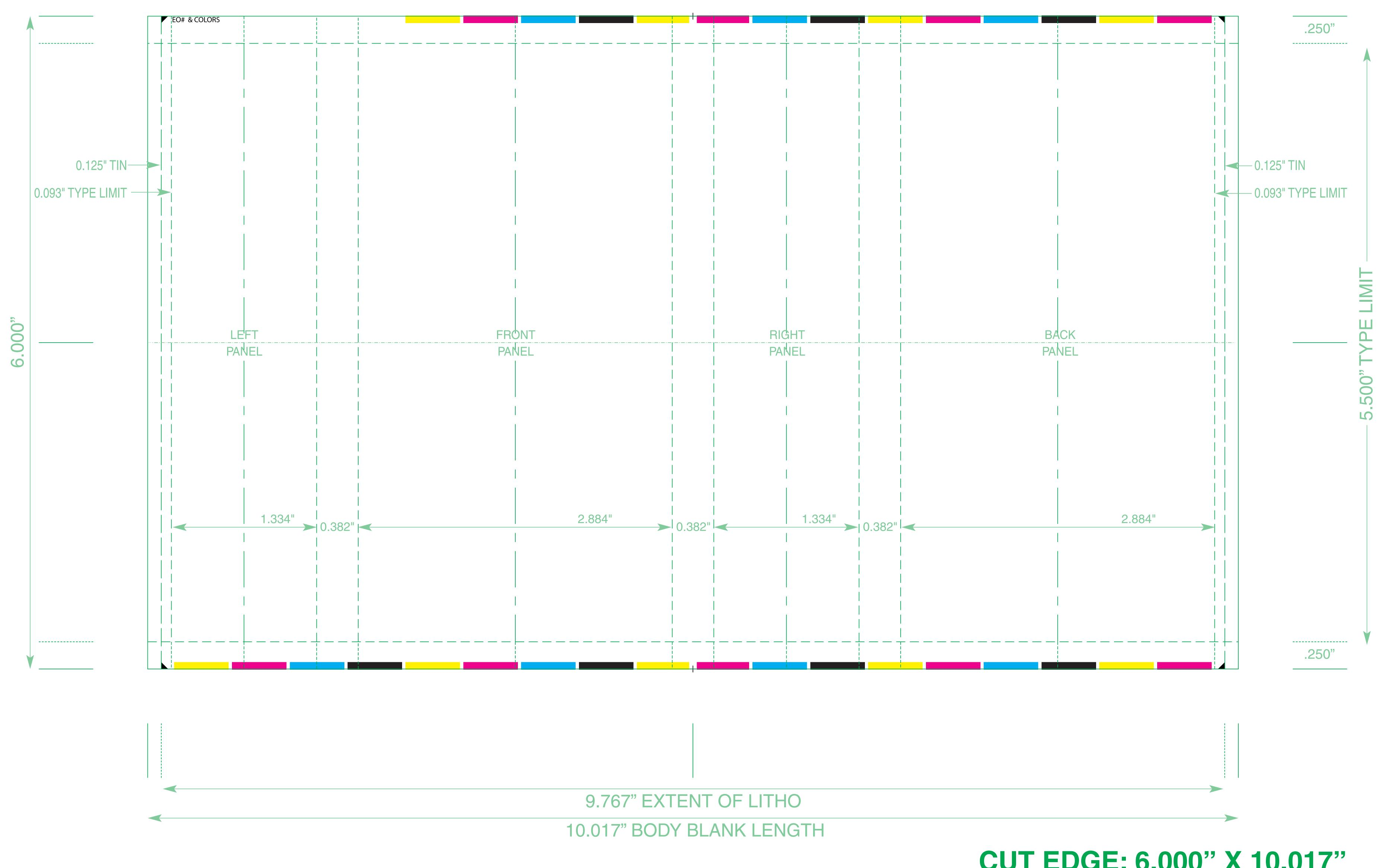
PINT "F" STYLE BODY WELDED SIDE SEAM @ 60° CUT EDGE: 6.000" X 10.017" **MASTER MARKS PRINTED AT 100%**
