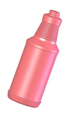
Nominal Capacity - 32 fluid ounces Overflow Capacity - 33.7 fluid Ounces Material - HDPE (Solvay B53-35H-011) or equivalent Neck Finishes - SPI "M" style 28-400 -28-410 and 38mm Cap Snap available Weight - 50 ± 3 grams
