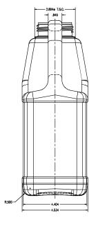
"REIKE" 63mm SCR. CAP #M0768 2 1/2 FULL TURNS OF THREAD, .167 PITCH SCALE: 2X
