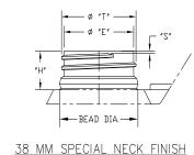
"T" DIM. 1.452 / 1.476 "E" DIM. 1.358 / 1.382 "H" DIM. .635 / .665 "S" DIM. .031 / .061 "I" DIM. (MIN.) .987 BEAD DIA. 1.524 +.022/-.012 THREAD TURNS 1-1/2 THREAD LEADS 6 PITCH .167
