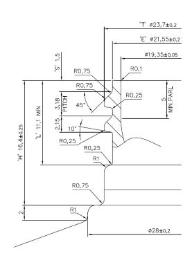
24mm S.P.I.410 'M' STYLE FINISH R.H.SINGLE START 8 T.P.I (0,125" PITCH) 1,5 TURNS OF FULL THREAD HELIX ANGLE 2' 34' MIN. THRO. BORE Ø18 @
