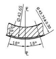
Thread's Detail on Parting Line (S=3:1)
