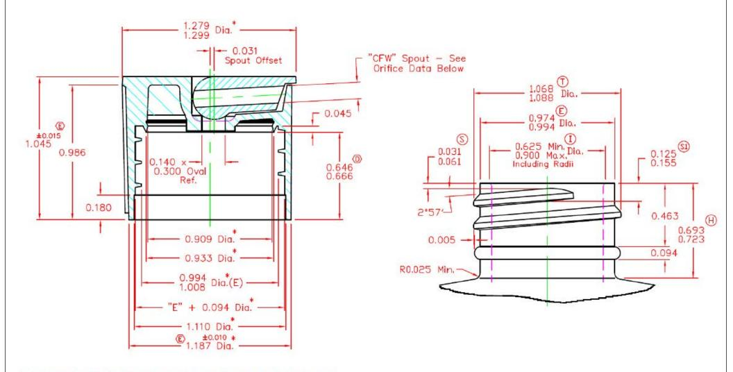
t Seal Type No. 1: Valve Seal (The most efficient provided bottle has proper "I" dimension)
