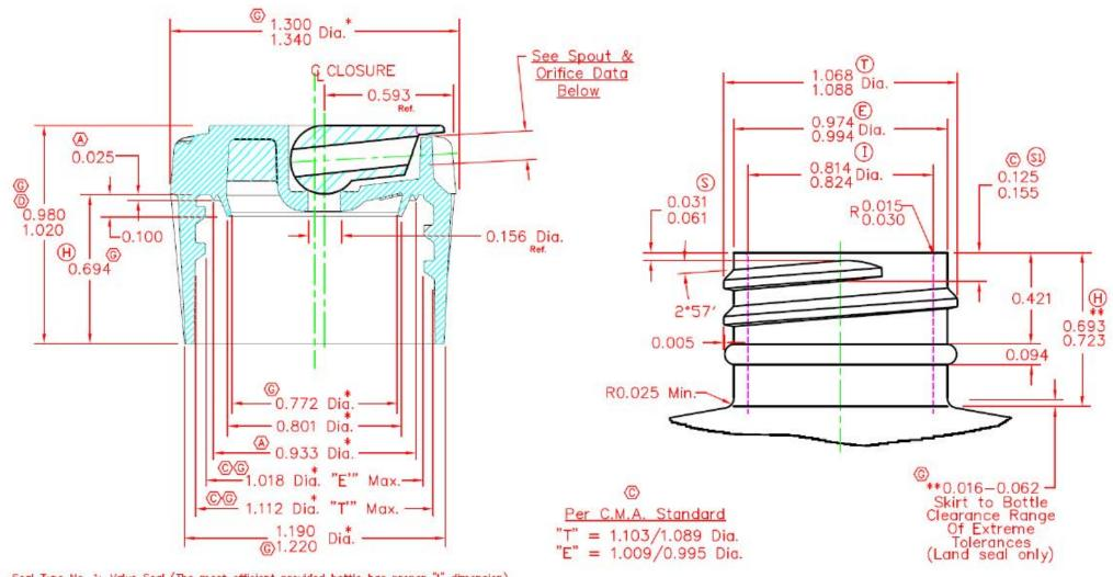
† Seal Type No. 1: Valve Seal (The most efficient provided bottle has proper "I" dimension) Seal Type No. 2: Land Seal ("I" dimension of bottle less critical than above)
