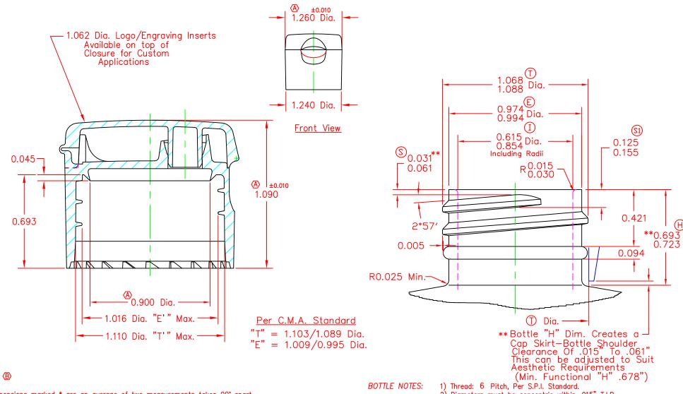
Dimensions marked \* are an average of two measurements taken 90° apart. GENERAL TOLERANCE NOT SHOWN OTHERWISE: ± .008
