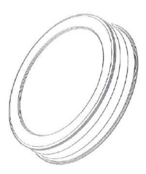
70-450 CT CAP "FTS" FLAT TOP STACKING PANEL LPD BUTTON WITH PLASTSOL LINER MATERIAL. 75# T-4, 55# DR-9 PULL DOWN VACUUM 8.0 IN. HG. MAX. WITH A VACUUM TETURN 2.0 IN. HG. MIN.
