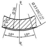
Thread's Detail on Parting Line (S=3:1)
