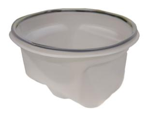
PRODUCT DESCRIPTION: The 5HD/CRDL/ONE-GAL is a rigid, durable, straight-sided, seamless, vacuum-formed cradle for keeping a can, up to 1-gallon in size, separated from the other contents of a 5-gallon plastic pail. This robust insert is molded from FDA-approved high-density polyethylene, thus it provides good resistance to many solvents. A contoured lip snaps over the top bead to prevent leakage between the insert and the pail wall. The ST is a short trim lip of 5/8".
