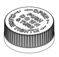
STATIC TORQUE RECOMMENDATION: 15-25 in-lbs requirement may vary depending upon container material, neck finish, and capping equipment
